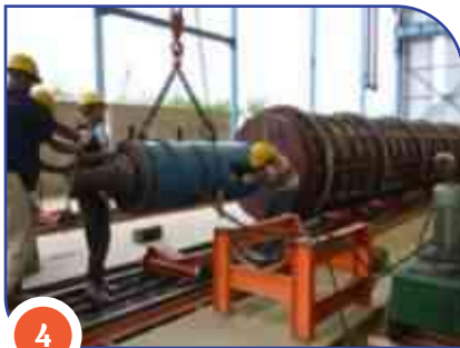
Penarikan Besi Prategang Prestressing Iron Withdrawal
