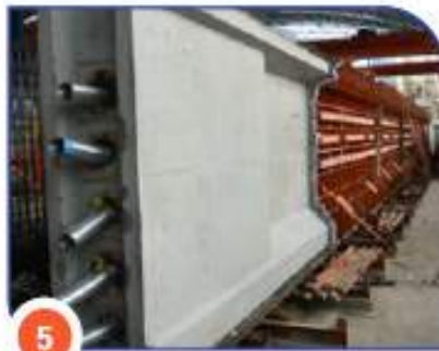
Pengecoran dan Pemasatan Beton Casting and Compaction of Concrete
